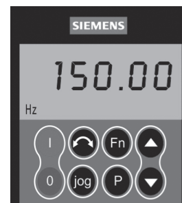
Fig. I — Siemens VFD Low Ambient Temperature Controller
